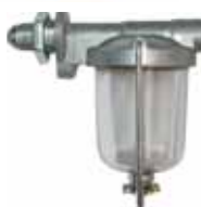
FUEL BOWL COMPLETE 29-31 09155 $73.00 Die cast body with heavy duty glass bowl seal and screen. excellent item.
